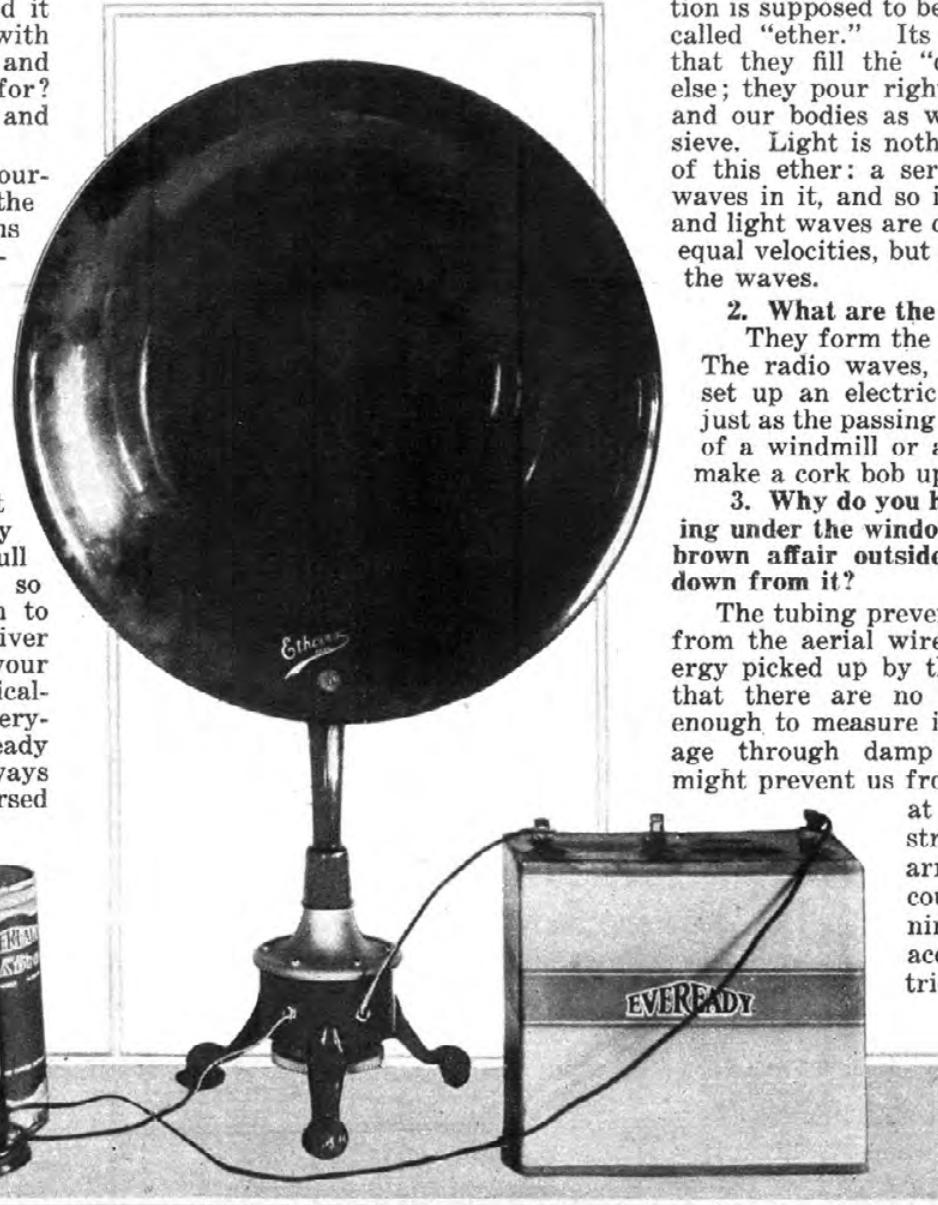
Here's a radio outfit, sketchy, but workable nevertheless. The loud speaker and "B" battery at the right form the real music and speech-making equipment. The vacuum tube and its filament battery in the center are simply the medium whereby the radio currents coming in from the left are permitted to increase or reduce the strength of the "B" battery current and thereby cause the speaker's diaphragm to give off intelligible sound waves
