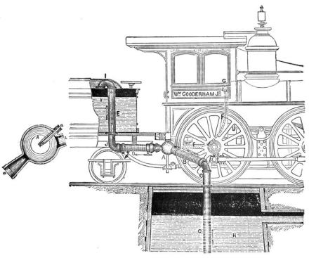
The injector, A, is a spherically shaped vessel, into which the water is drawn from the source of supply, through a four-inch pipe, by the vacuum formed within the vessel, and from which it is forced through another four-inch pipe, into the Tender, by the action of the steam drawn from the boiler.
