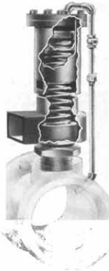
Relief Valve with Sleeve for connecting to water main
