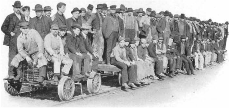
Showing one of the practical uses of the Section Motor Car No. 14. Load, 86 men; total weight including car, 17,351 pounds, at a speed of five miles per hour on level track. Send for special Motor Car Catalogue No. 480.
