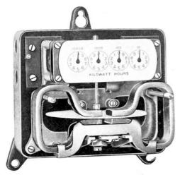
Thomson High Torque Induction Wattmeter With Cover Removed
