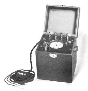
CASE WITH COVER REMOVED SHOWING CORD AND SWITCH FOR CONTROLLING THE METER
