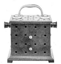
MULTIPLIER FOR PORTABLE VOLTMETERS AND AMMETERS
