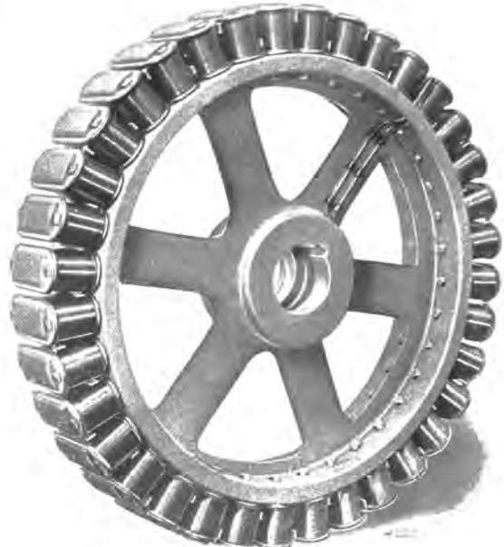
REVOLVING FIELD WITH STRIP WOUND COILS
