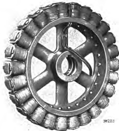
Fig. 5. REVOLVING FIELD—WITH WIRE WOUND COILS
