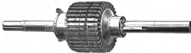
CVC ARMATURE CORE ASSEMBLED ON SHAFT
