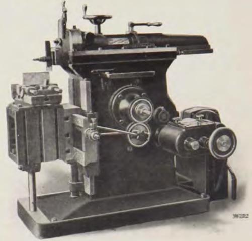
15-IN. CINCINNATI MILLING MACHINE CO. SHAPER DRIVEN BY KT-4, 3 H.P., 1800 R.P.M. INDUCTION MOTOR
