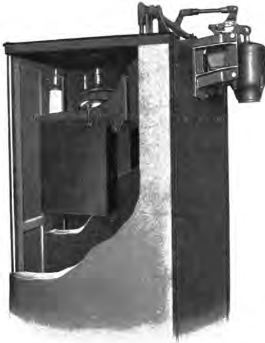
Fig. 6 SOLENOID-OPERATED T.P.S.T. FORM K-12 OIL BREAK SWITCH OF 3 SINGLE-POLE ELEMENTS MOUNTED IN CONCRETE CELL
