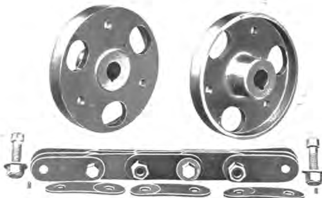
Fig. 2 DISASSEMBLED VIEW OF LEATHER LINK FLEXIBLE COUPLING
