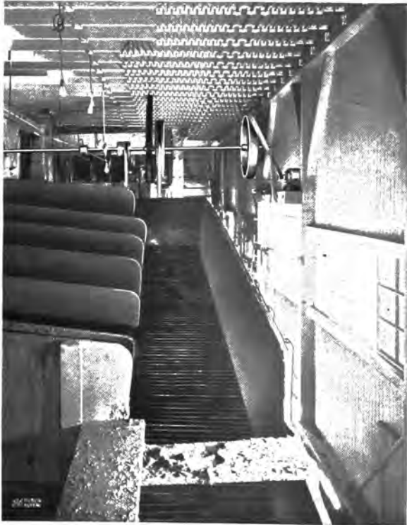
INTERIOR OF YUBA NO. 12 SHOWING GOLD SAVING TABLES AND OVERHEAD WIRING FOR THE VARIOUS MOTOR CIRCUITS
