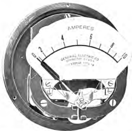
INTERIOR OF SWITCHBOARD AMMETER, TYPE R-6
