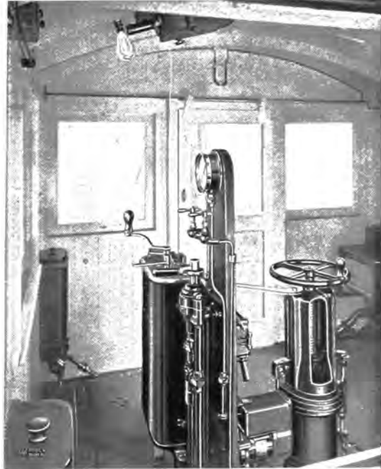
INTERIOR OF CAB SHOWING ARRANGEMENT OF CONTROL APPARATUS INCLUDING COMBINED HAND AND AIR BRAKE CYLINDER
