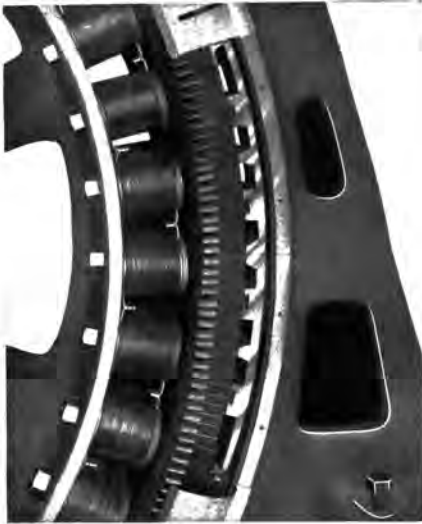
Fig. 1 SECTION OF ALTERNATOR SHOWING METHOD OF DOVETAILING CORE LAMINATIONS TO STATOR FRAME
