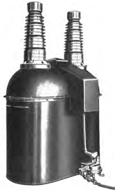
SINGLE ELEMENT OF FORM K-15, 100 AMPERE 110,000 VOLT OIL BREAK SWITCH PNEUMATICALLY-OPERATED
