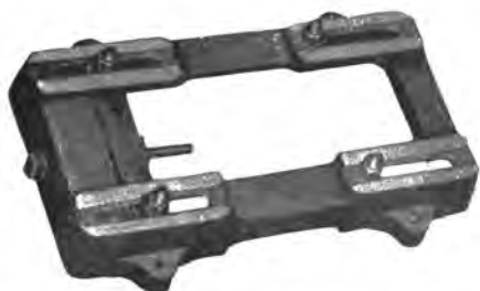
SLIDING BASE SHOWING FASTENING AND ADJUSTING BOLTS
