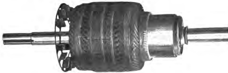
CVC GENERATOR ARMATURE
