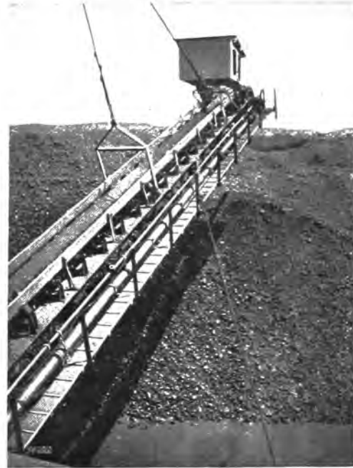
STACKER OF DREDGE EL ORO NO. 3 SHOWING HOUSE CONTAINING THE STACKER MOTOR
