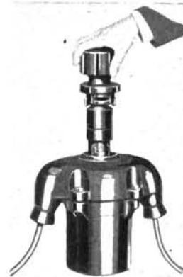
INSERTING THE FUSE CARRIER. A SLIGHT TURN LOCKS IT, AND A 90 DEG. TURN CLOSES THE CIRCUIT UNDER OIL
