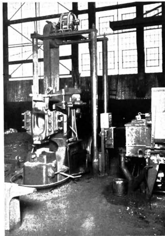
7 1/2 H.P. TYPE I FORM K MOTOR DRIVING 300 POUND HAMMER IN BLACKSMITH'S SHOP
