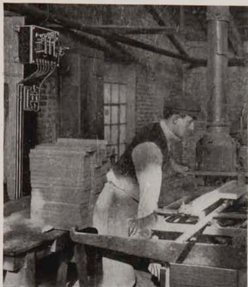
FOR MACHINERY IN GENERAL Mount the Starter on a Wall or Post, the Push Button on the Machine. Convenience of Control Increases Production
