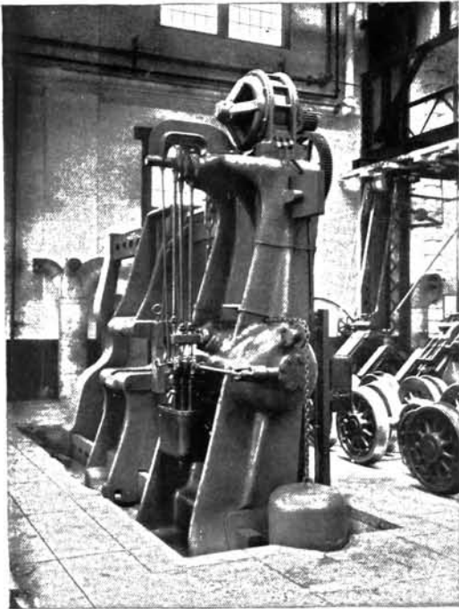
90 IN. 600-TON WHEEL PRESS, OPERATED THROUGH GEARING BY 25 H.P., 750 R.P.M., 550 VOLT, FORM K INDUCTION MOTOR
