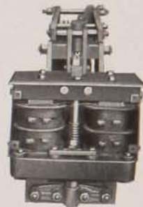
End view of brake with cover removed, showing solenoid coils and connections
