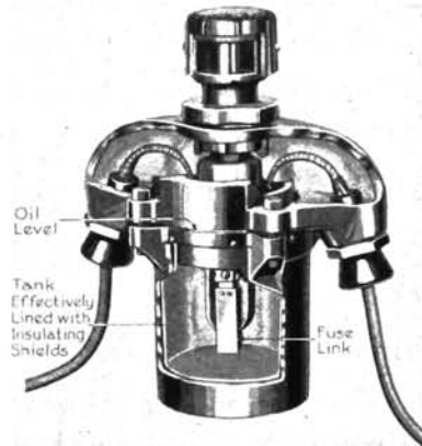
POLE TYPE CUTOUT, SECTIONAL VIEW
