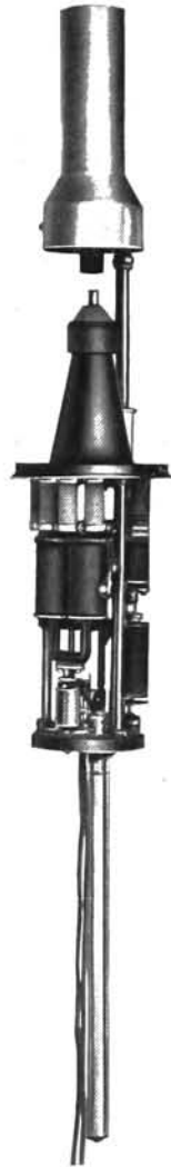
Complete Mechanism Showing Tube for Lower Electrode
