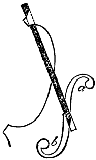
FIG. 155.—Method of raising the wing a of the f hole.
